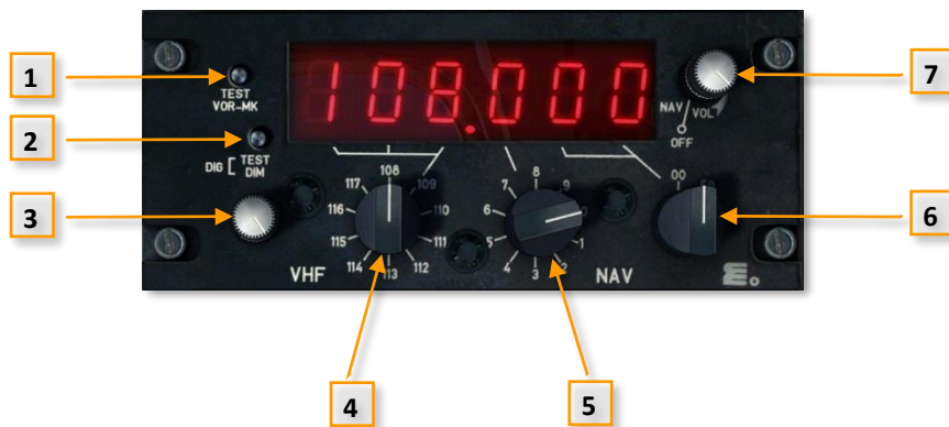
Figure 3-73 VOR/ILS control panel
