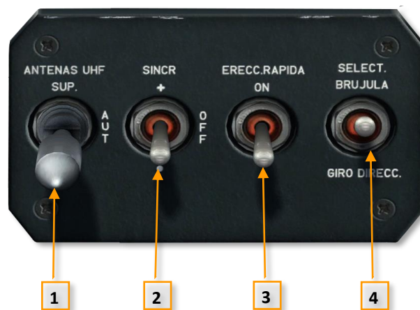
Figure 3-79 TARSYN control panel
