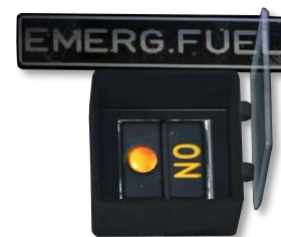
Figure 9-12 Emergency Fuel Switch
