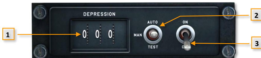
Figure 9-37 Optical Sight Control Unit
