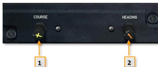
Figure 3-78 HSI remote control panel
