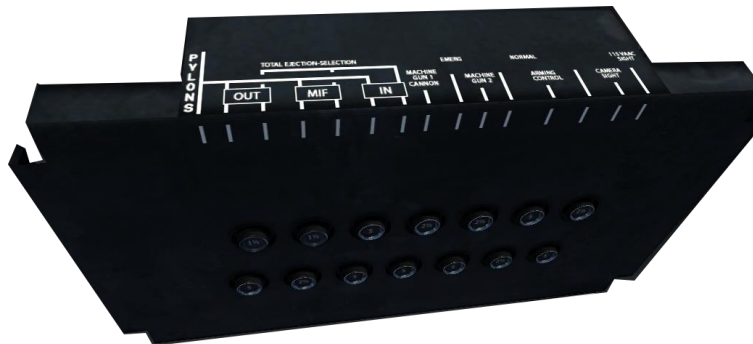
Figure 9-10 Armament Circuit Breaker Panel
